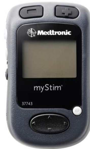
Spinal cord remote controller. Image courtesy of Medtronic Inc.
